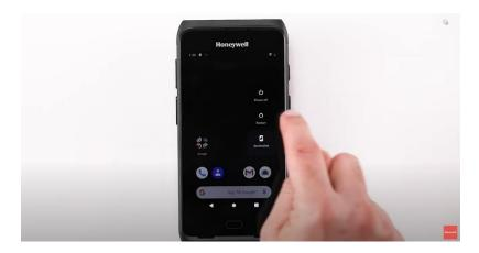
3. With the device off press and hold the **Volume Down** button, while doing so press the **Power b**utton.
